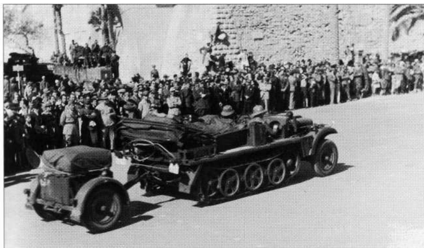
A 1-ton half-tracked Demag D7 SdKfz 10 with trailer on which the tactical insignia of a Panzerjäger unit is just visible. That makes it very likely part of the Panzerjäger Abteilung 39. (Carlo Pecchi Collection)
