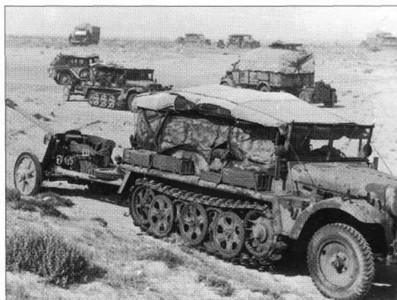
A Panzerjäger Zug during a moment of rest, in the foreground the usual Demag D7 SdKfz 10 towing a 50mm Pak 38. The fact that the vehicles only have a coat of sand over their European dark-grey colour, and also the presence of Pak 35/36 37mm guns towed by other Demags, suggests the photo was taken in early 1941 and that it probably shows elements from Panzerjäger Abteilung 39 . Note the use of the Zeltbahn (camouflage sheet) as a sun shield. (Carlo Pecchi Collection)
